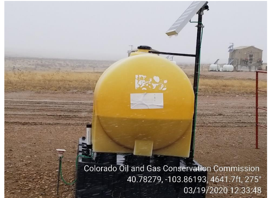
Photo 8 – Chemical Tank Labels have faded
