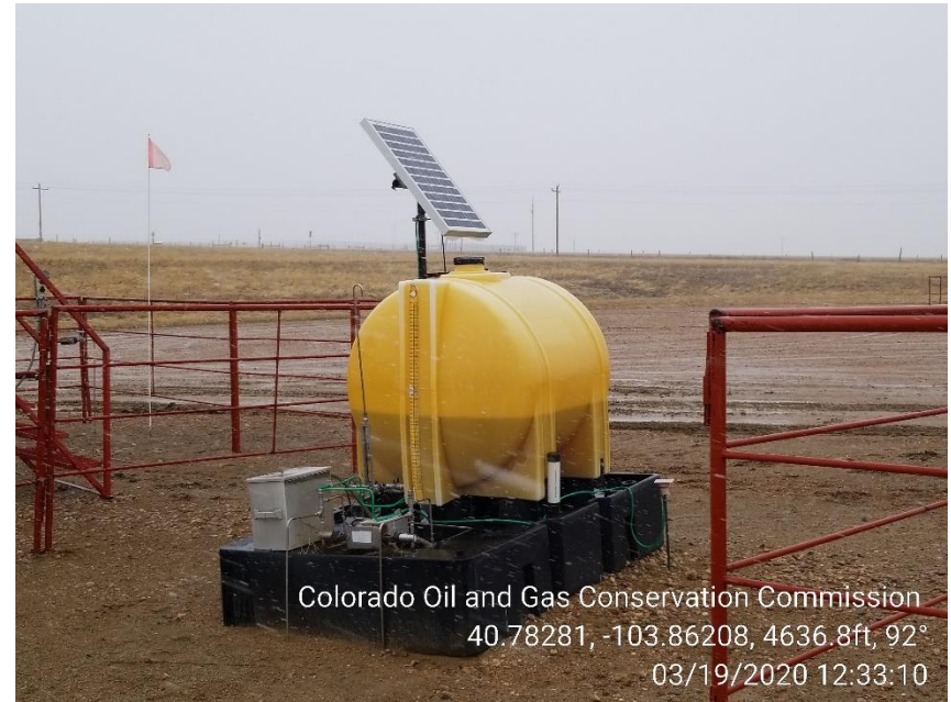
Photo 6 – Chemical Tank missing Labels
