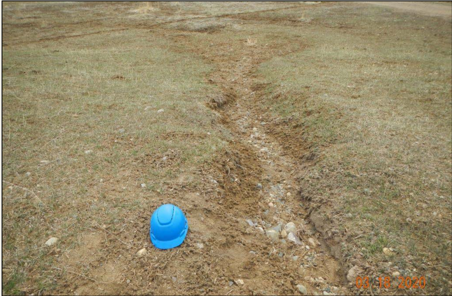
Photo 3. View of erosional channel approximately 2 feet wide and 1 foot deep, forming within the southwestern corner of the project area. Hard hat in place for scale reference.
