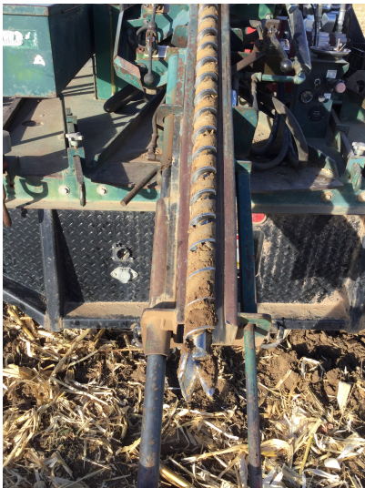
Photo 3. Collected Soil Core to Depth of 18', Dry. December 11, 2017. Location: 40.38580, -104.80817
