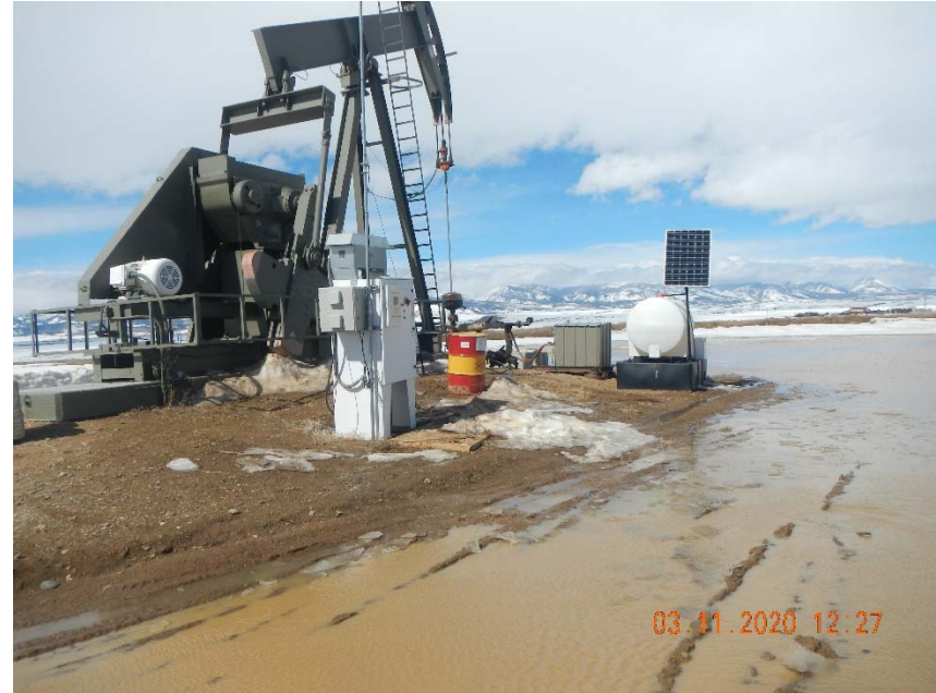
Photo 2. Container at wellhead without secondary containment.
