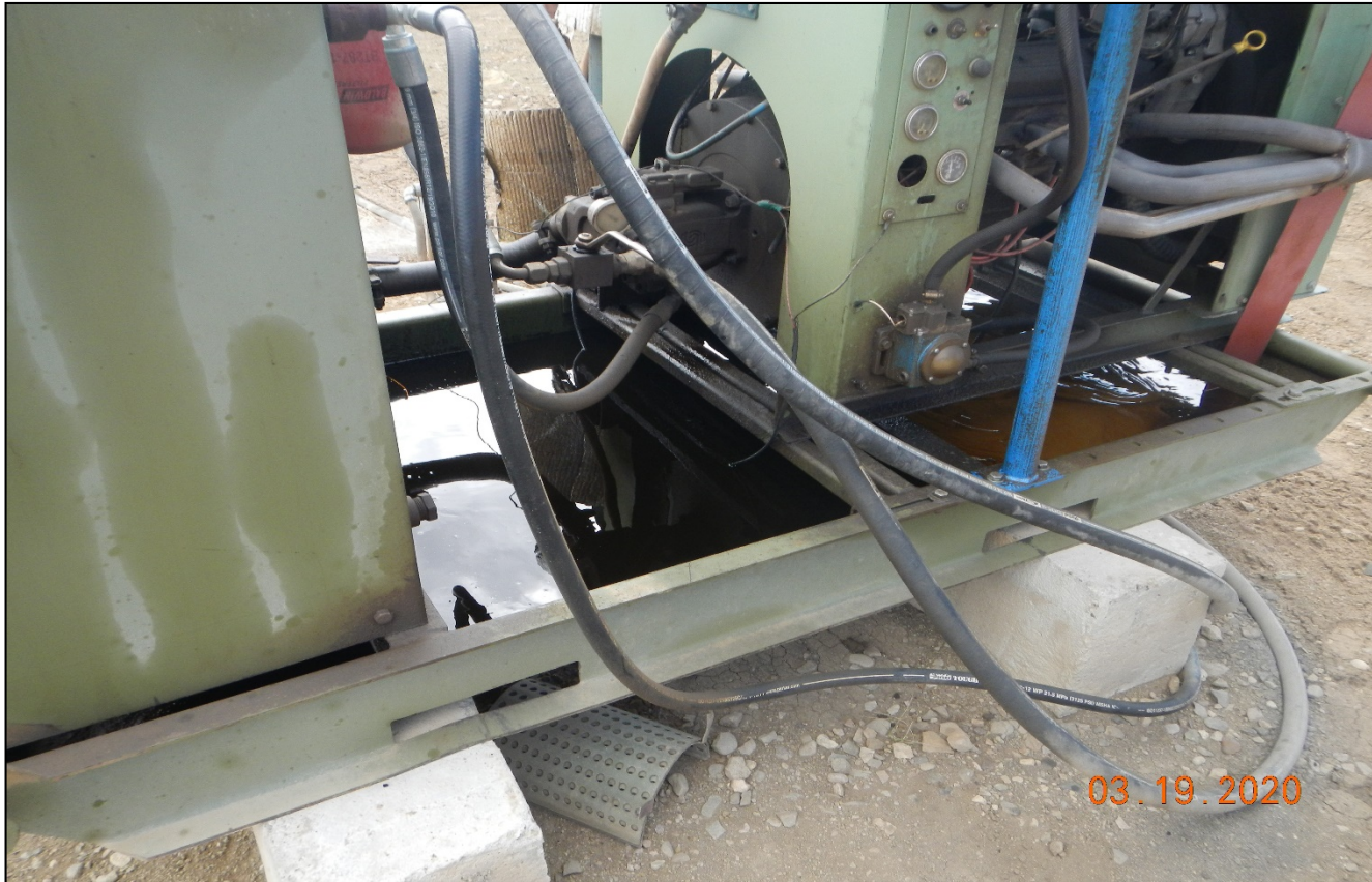
Photo 3. There is oil on the engine skid and on soil that needs to be cleaned up.
