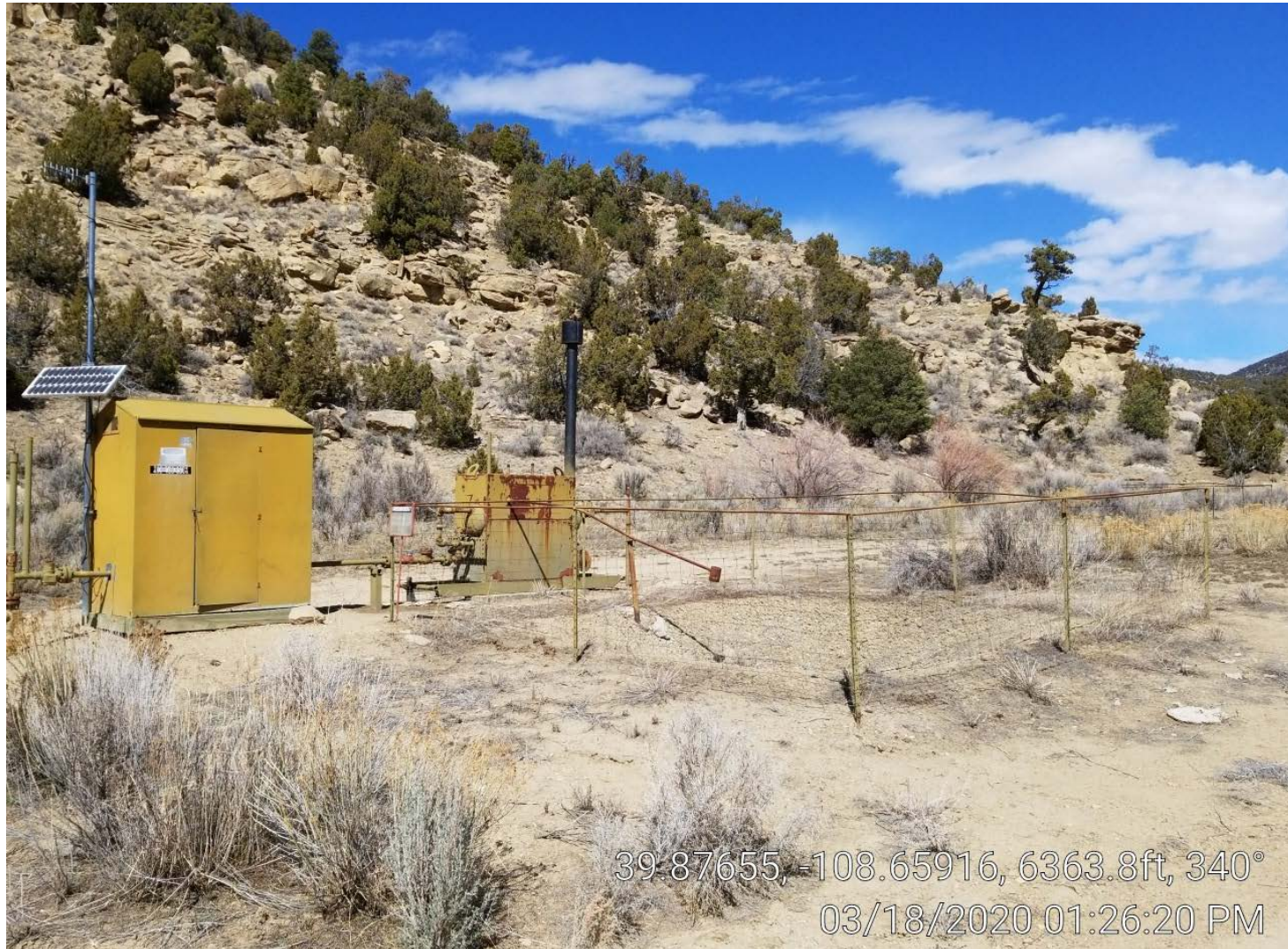
Photo 2. Meter building, separator, and separator pit.
