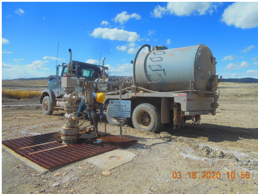
Injection wellhead
