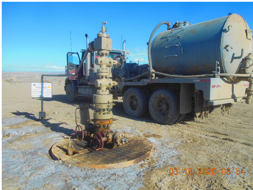
Injection wellhead
