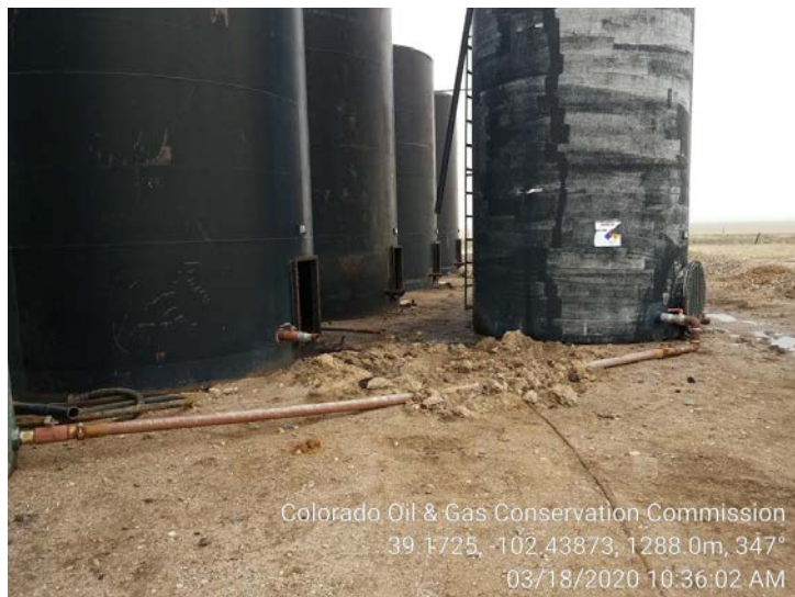
1. Tanks with Manhole covers removed
