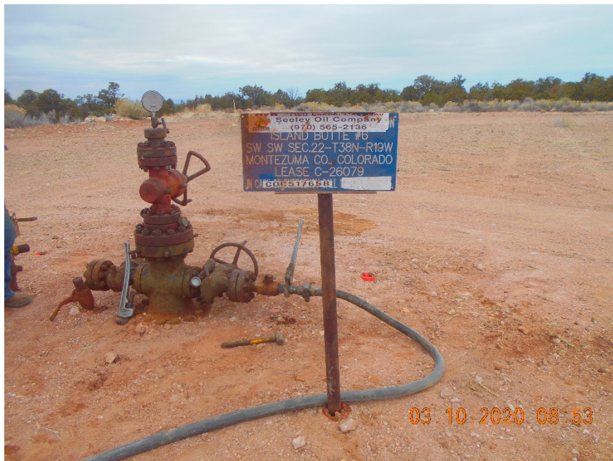
Temporarily abandoned wellhead with sign. MIT to maintain SI/TA status.
