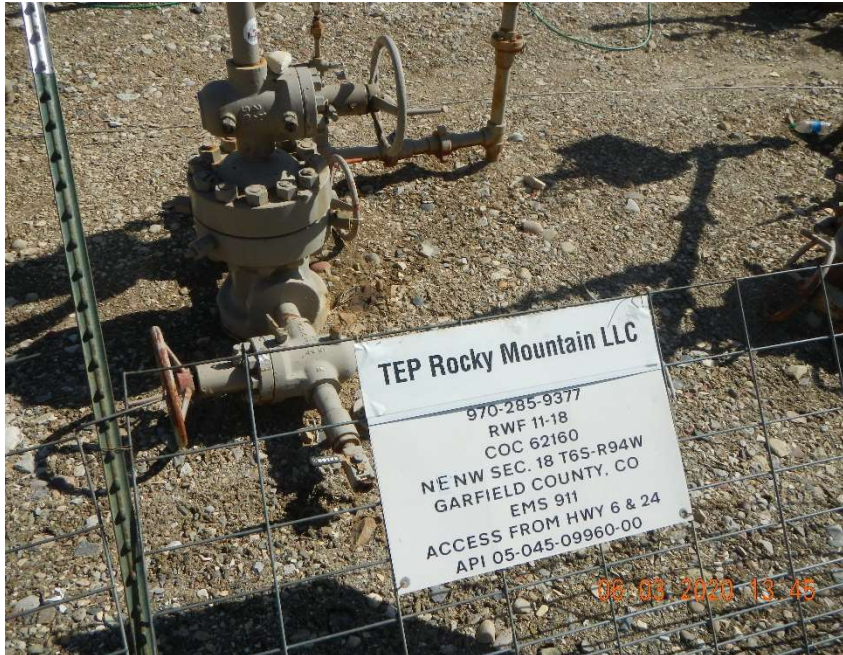
Localized accumulation of oily waste around wellhead.
