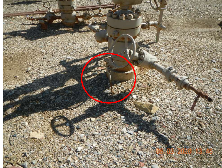
1-inch riser adjacent to RWF 312-18 wellhead.
