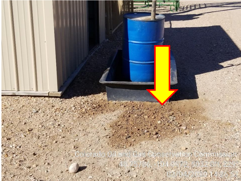
Photo 5 – Stained Soil at SE corner of Pumping Unit
