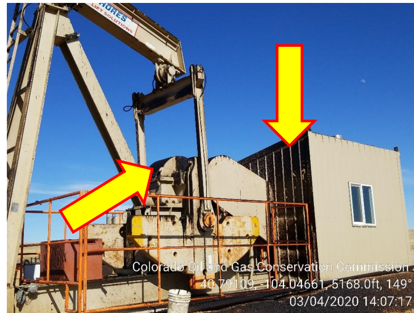
Photo 2 – Oil sprayed over Pumping Unit
