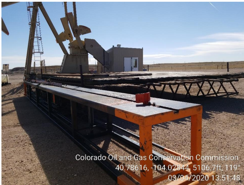
Photo 3 – Unused Tubing String and Pipe Rack
