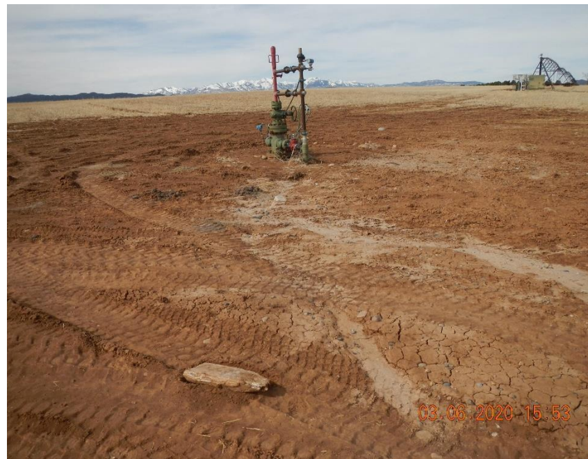
Drainage pattern with discolored soil extending SE from well head.
