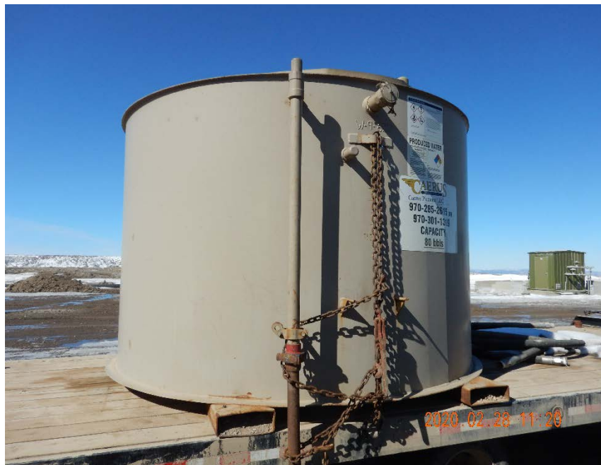
Photo #35 – AST from previous photo is labeled to contain Produced Water with a capacity for 80 bbls.
