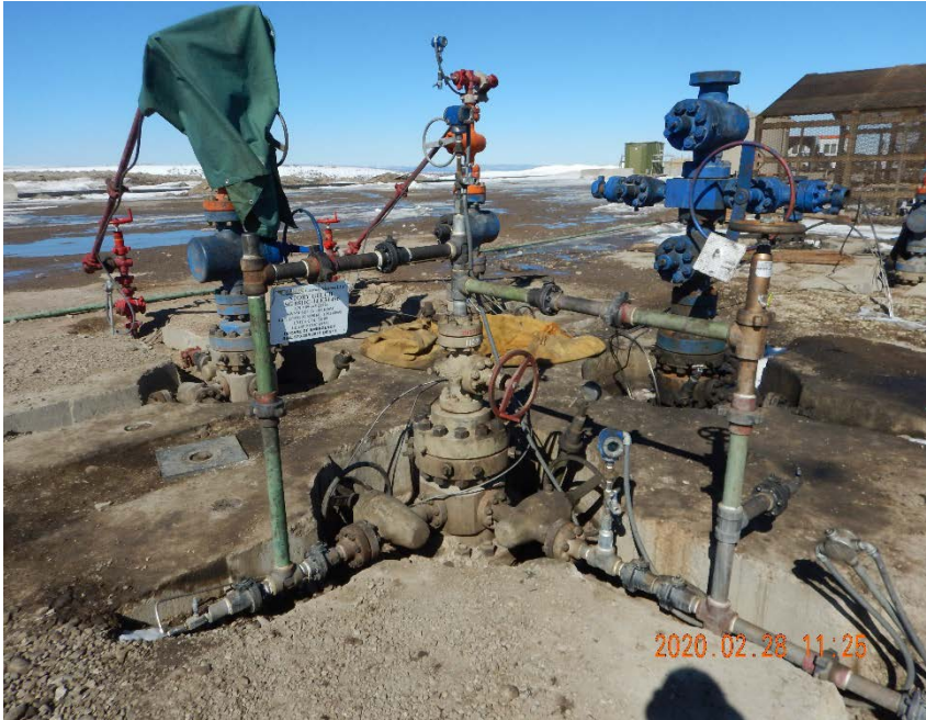
Photo #19 – Localized accumulations of hydrocarbon staining on cement and soil in vicinity of API #05-045-21928.
