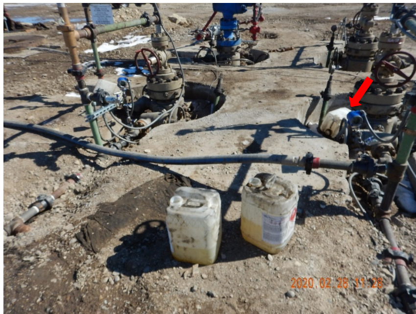
Photo #33 – Localized accumulations of oil-stained soil and chemical storage containers with trash stored on west side of API #05-045-21905. Note overturned chemical storage container marked by red arrow.
