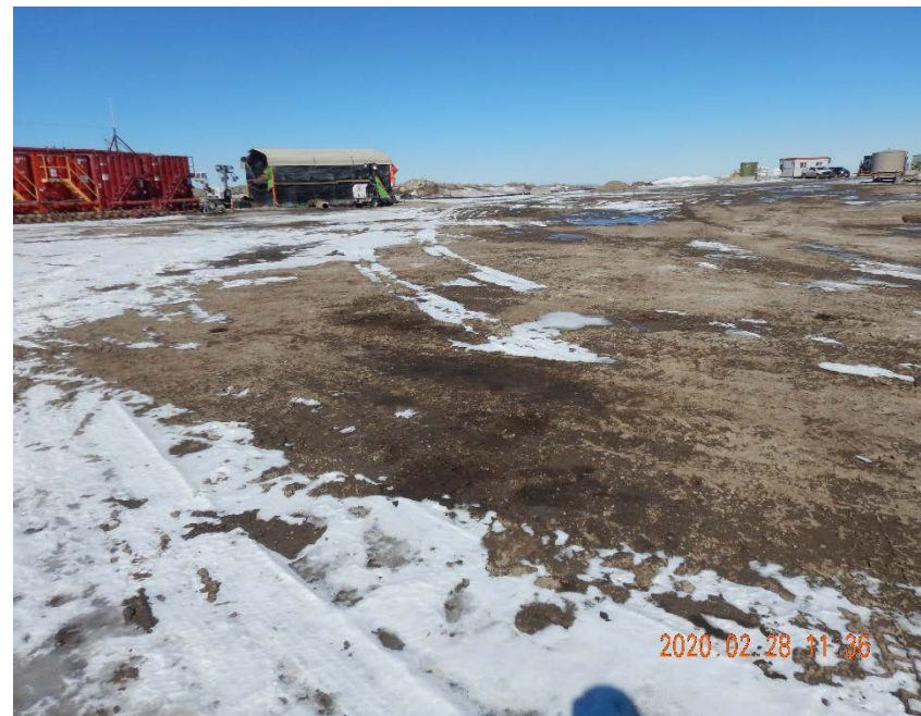
Photo #32 – Localized accumulations of oil-stained soil and impacted fluids on south side of pad.
