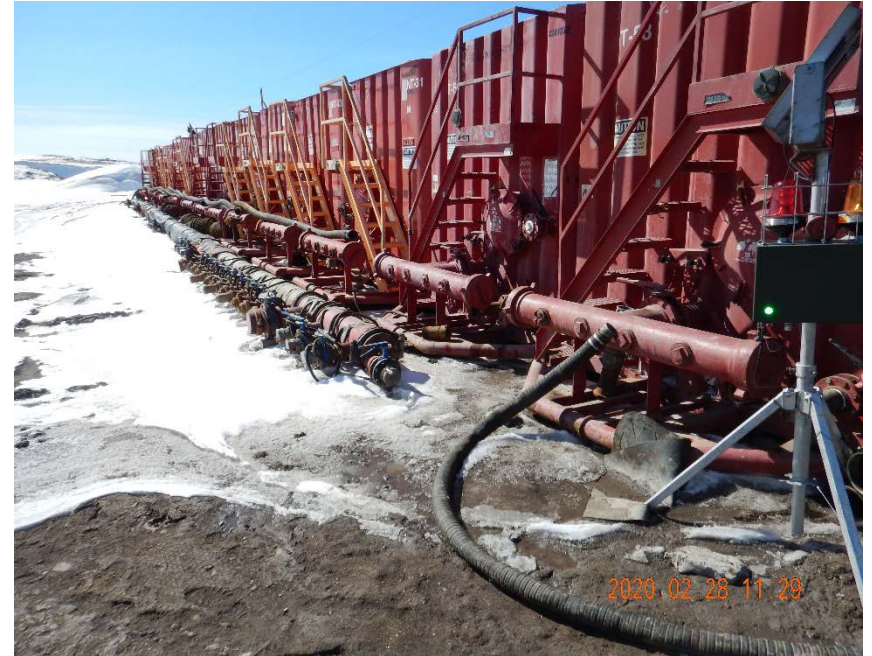
Photo #38 – View of frac tanks from northeast. Frac tanks lacked content labels and NFPA placards on inspection date.
