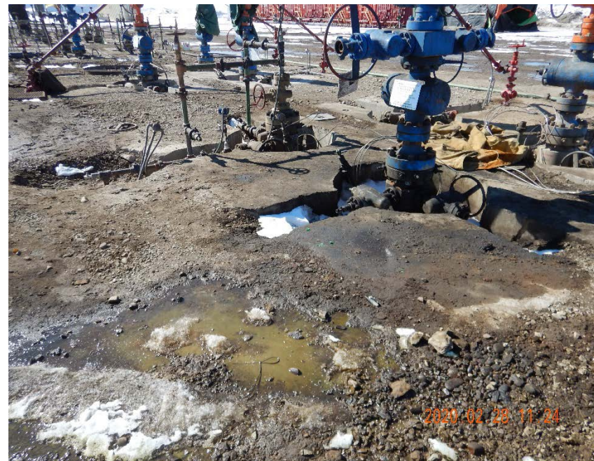
Photo #18 – Localized hydrocarbon staining, impacted fluids, and stained soil located west of API #05-045-21923.
