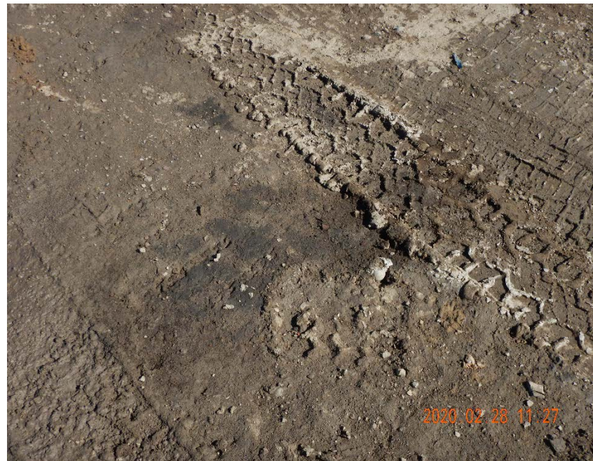
Photo #24 - Localized accumulations of oil-stained soil located west of wellheads (3).
