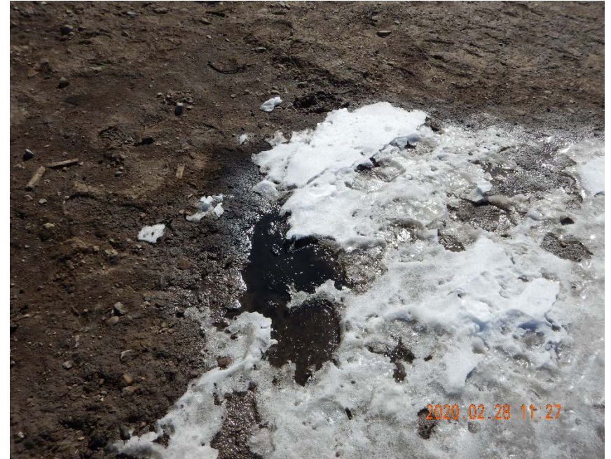
Photo #26 - Localized accumulations of oil-stained soil located west of wellheads (5).
