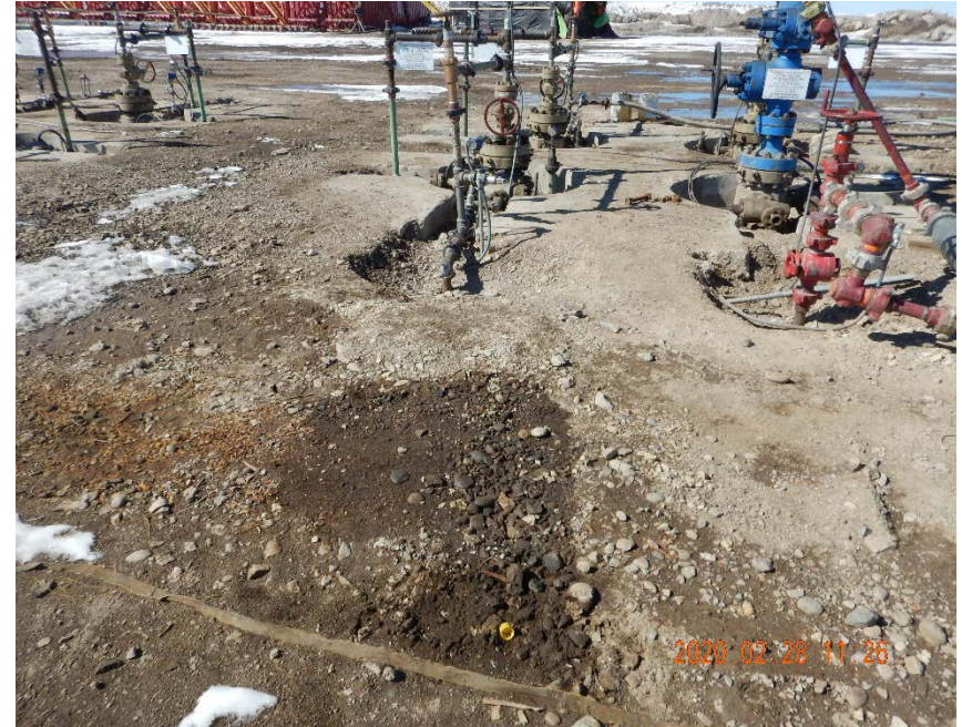
Photo #20 – Localized accumulation of oil-stained soil east of API #05-045-21919.
