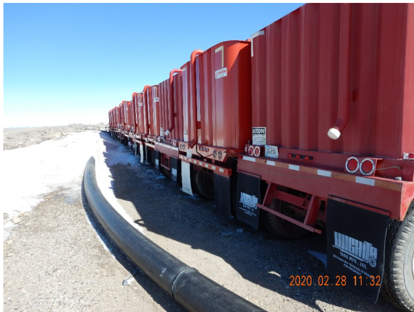
Photo #39 – View of frac tanks from southwest. Note absence of secondary containment device.
