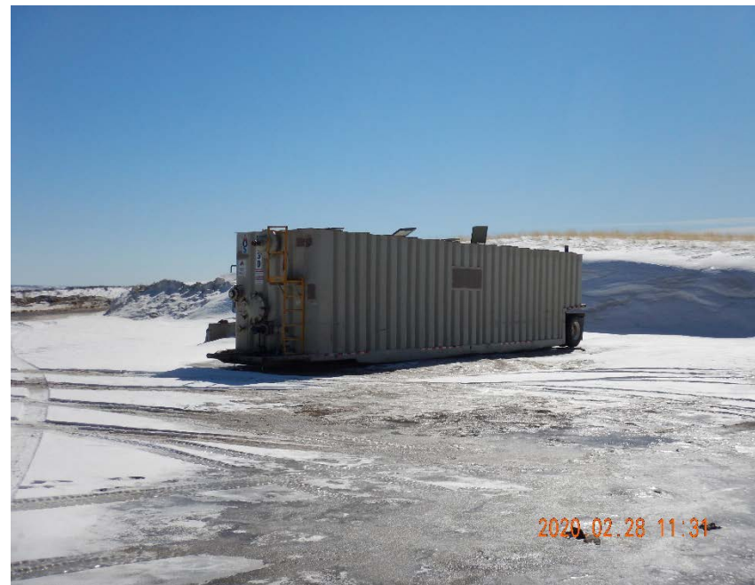
Photo #40 - Additional frac tank located on south side of pad also lacked secondary containment device on inspection date.
