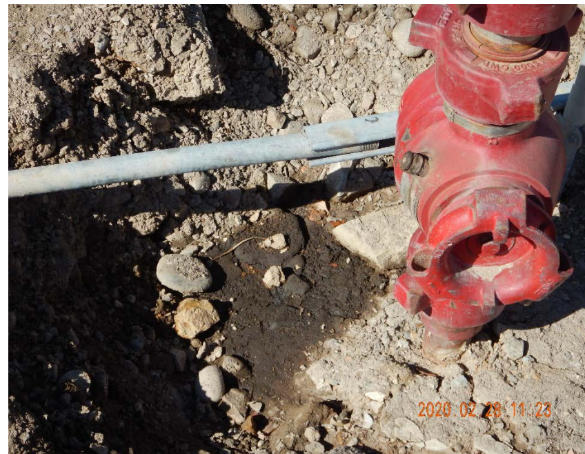
Photo #16 – Localized accumulation of oil-stained soil on east side of API #05-045-21909.
