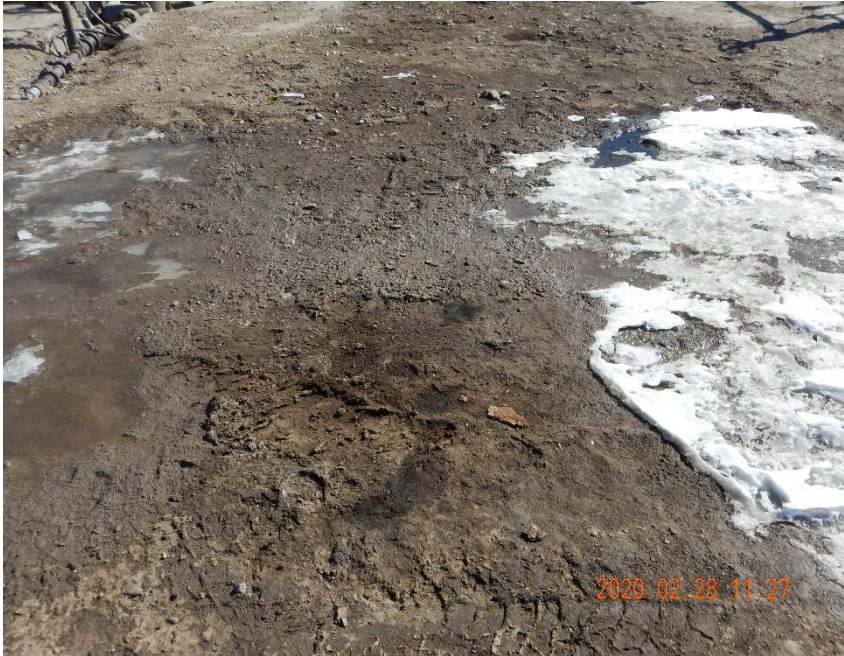
Photo #25 - Localized accumulations of oil-stained soil located west of wellheads (4).
