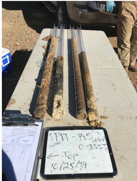
Photograph 2: Impacted soil observed at the center borehole at the Carl Allen 6 pad, Pit 17, COGCC ID 100688. Note the black staining present at approximately 6 ft bgs, second core from the left.
