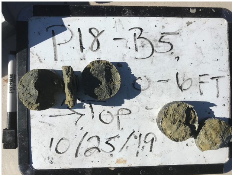
Photograph 2: Bedrock (siltstone) encountered at the Carl Allen 7 pad, Pit 18, COGCC ID 100623.
