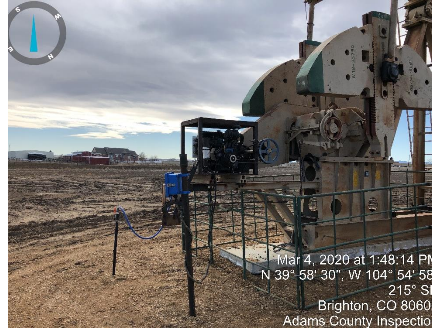
Photo #2 pulley guard missing from pump motor
