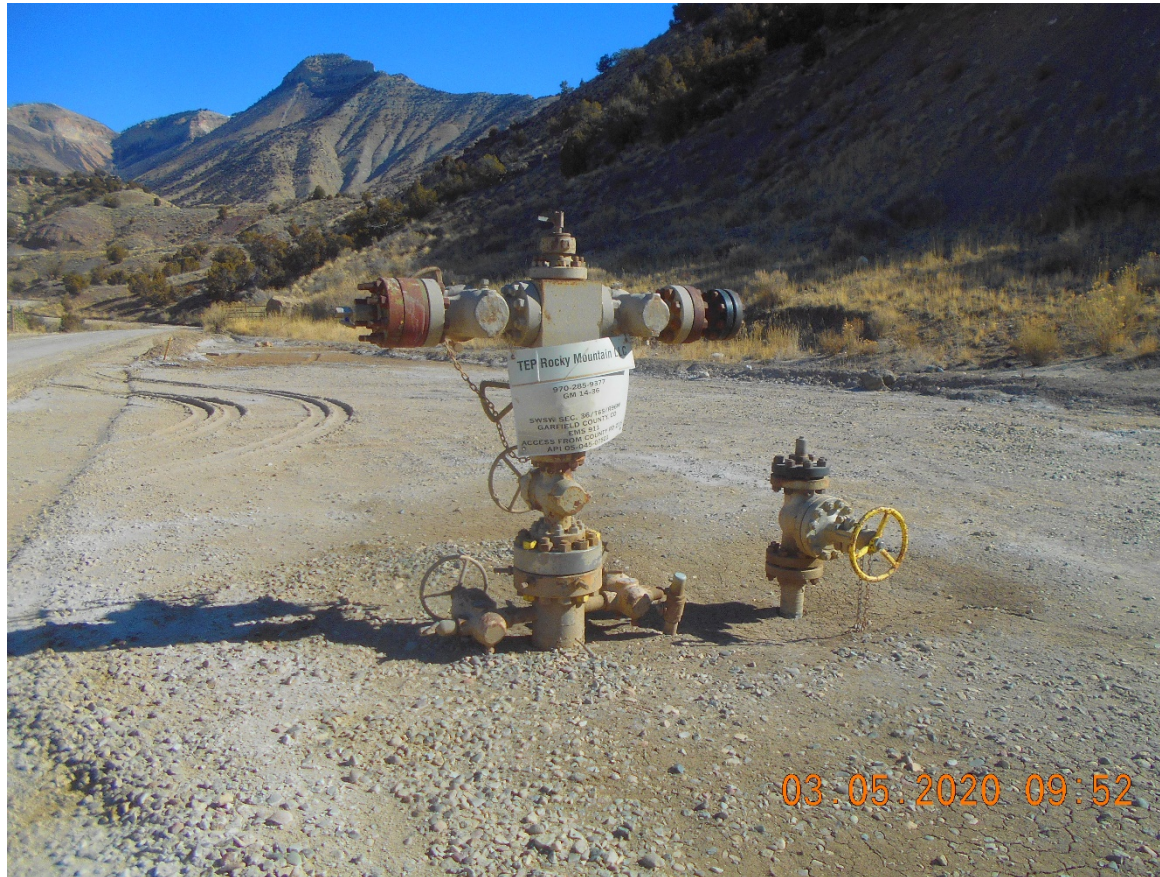
Injection wellhead. Temporarily abandoned.
