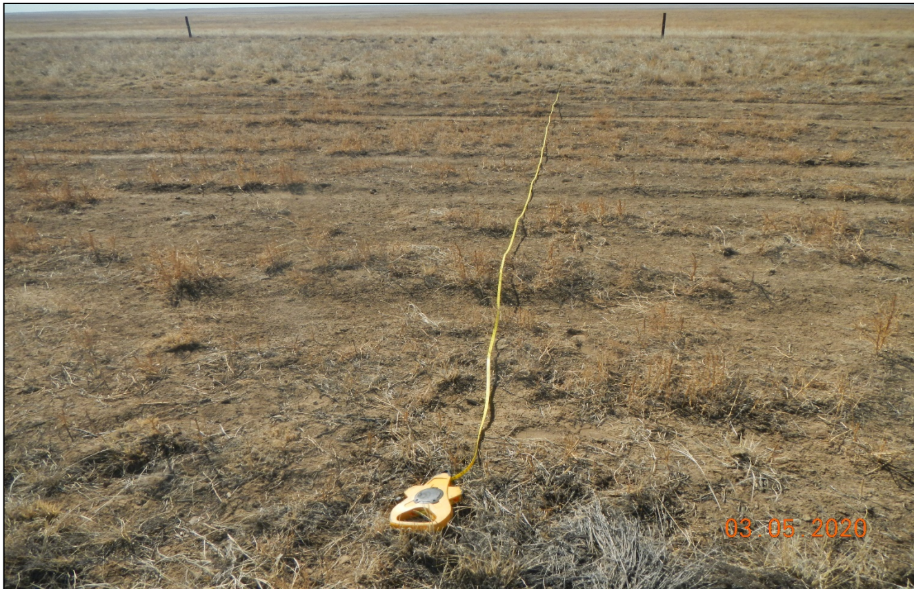
Photo 4. The disturbance of the access road was measured to be approximately 50 feet wide.
