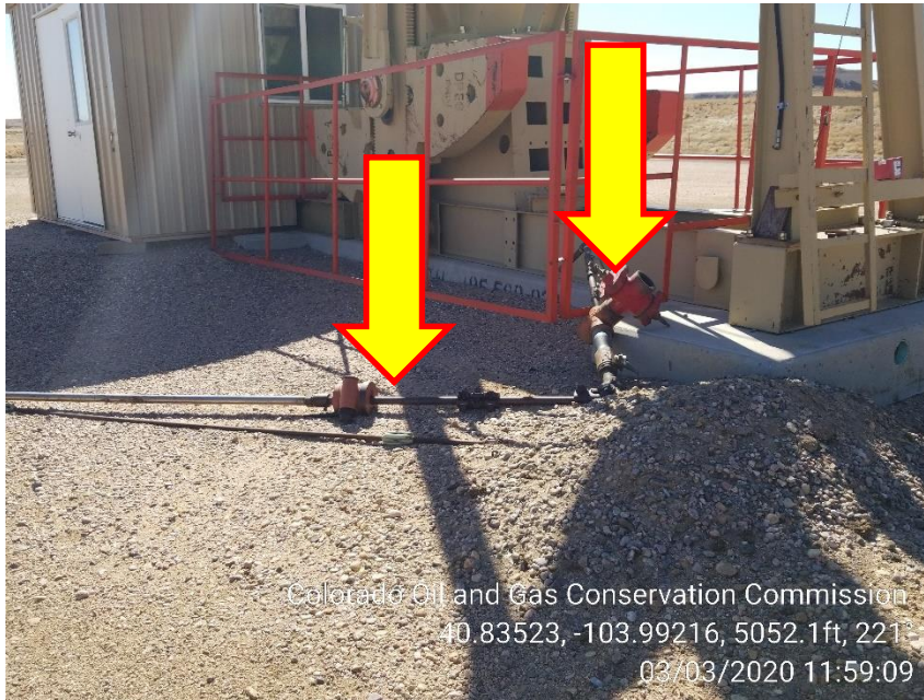
Photo 5 – Unused Polish Rod and wellhead parts
