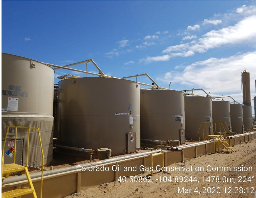
Photo 25: Tank Battery
