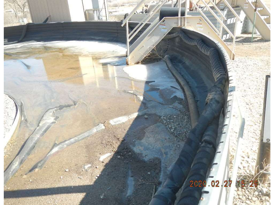
Unused equipment within the tank battery secondary containment.
