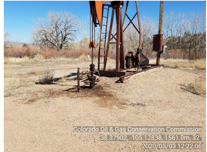
PHOTO 4: IT APPEARS THAT WELLHEAD IS LEAKING PRODUCED OIL, AREA OF IMPACTED SOIL APP. 6' BY 3' AROUND WELLHEAD. Securely fasten all valves, pipes, and fittings to ensure good mechanical condition, inspect at regular intervals and maintain in good mechanical condition per Rule 605.d. Properly treat or dispose of oily waste in accordance with 907.e. ACTION REQUIRED IMMEDIATELY AS CA DATE FROM PRIOR INSPECTION HAS PAST.
