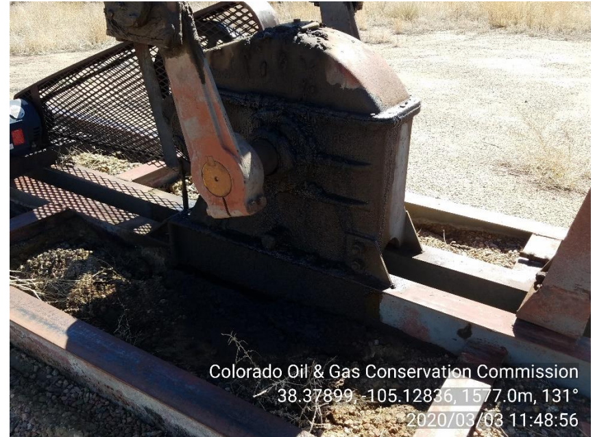
PHOTO 12: APPEARS THAT GEAR BOX ON PUMPJAKE IS LEAKING, THERE IS AN AREA OF IMPACTED SOIL BENEATH GEARBOX. Securely fasten all valves, pipes, and fittings to ensure good mechanical condition, inspect at regular intervals and maintain in good mechanical condition per Rule 605.d. Properly treat or dispose of oily waste in accordance with 907.f. ACTION REQUIRED IMMEDIATELY AS CA DATE FROM PRIOR INSPECTION HAS PAST.
