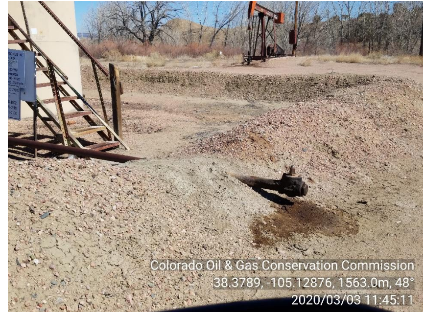
PHOTO 10: LOADOUT LINE IS PLUMBED OUTSIDE SECONDARY BMP. THERE IS AN AREA OF IMPACTED SOIL OUTSIDE OF BURM) APP. 1' BY 2' AROUND LOADOUT. INSTALL SECONDARY BMP TO PREVENT OILY WASTE FROM MIXING WITH STORM WATER PER RULE 1002.f. Properly treat or dispose of oily waste in accordance with 907.e.
