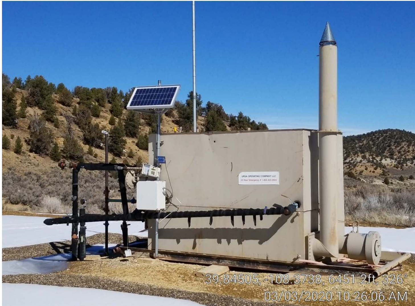
Photo 3. Horizontal separator.
