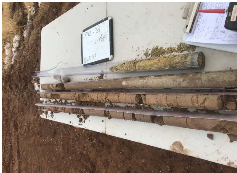
Photograph 1: Typical lithology observed at perimeter boreholes at the Jacks Draw 2 pad, Pit 12, COGCC ID 100620.
