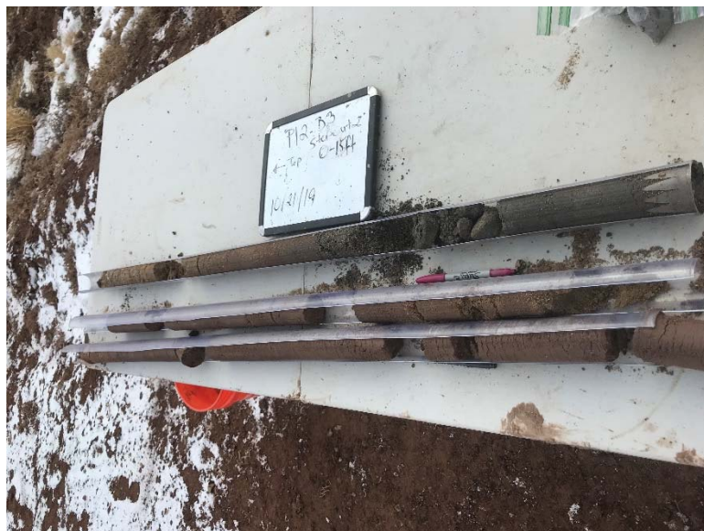
Photograph 2: Impacted soil observed at the Jacks Draw 2 pad, Pit 12, COGCC ID 100620. Note the black staining present at approximately 13-15 ft bgs (top core, to the right).
