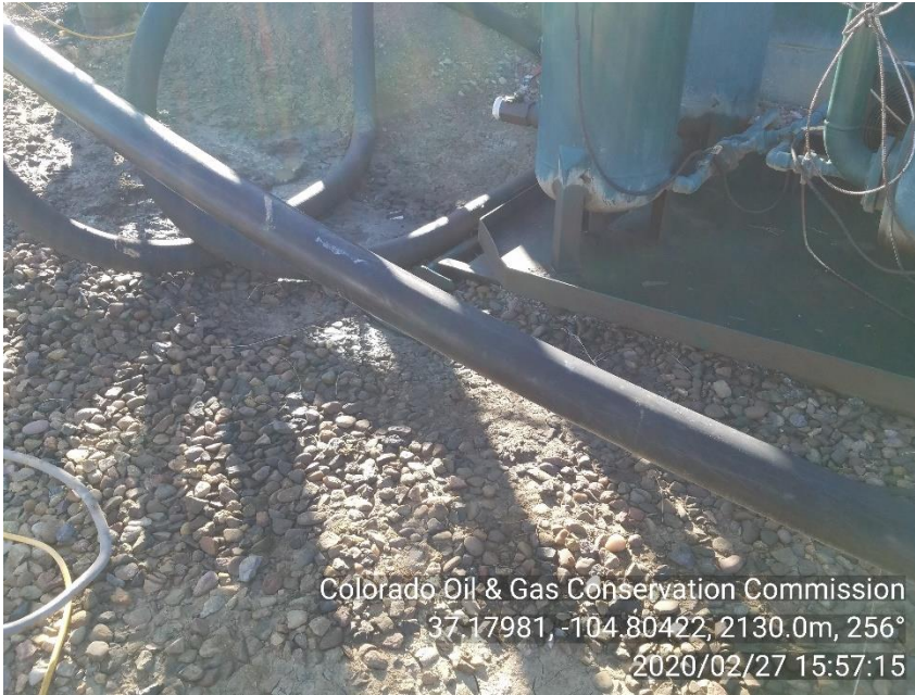
PHOTO 11: IMPACTED SOIL ALL AROUND AND UNDER COMPRESSOR SKID. Conduct maintenance on equipment, cleanup stained material and review self inspection processes. CA DATE 3-3-20.
