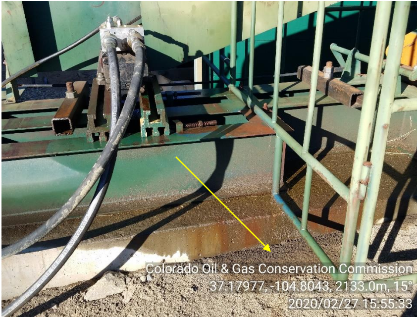
PHOTO 9: SOIL APPEARS TO BE CONTAMINATED FROM LEAKING HYDRALIC OIL. Conduct maintenance on equipment, cleanup stained material and review self inspection processes. CA DATE 3-3-20.
