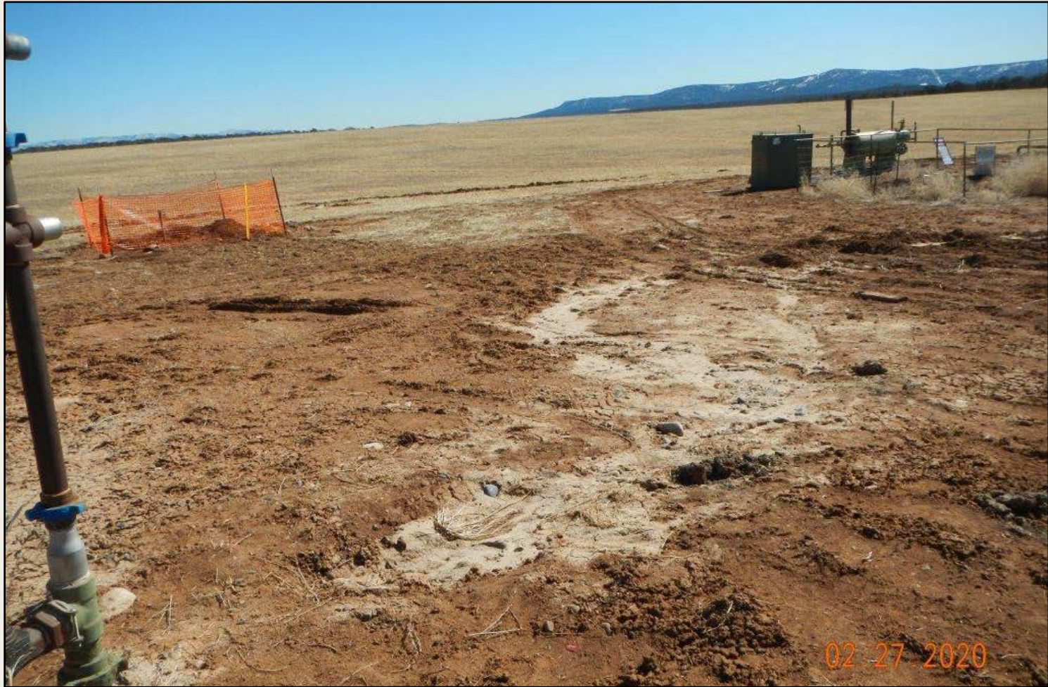
Photo 4. View of what appears to be release with discolored soil flowing toward southeast. Orange fencing surrounds an excavation area.
