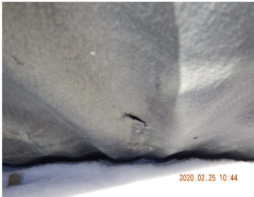
Photo #13 – Additional hole in lower tank battery liner
