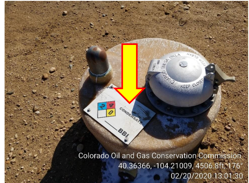
Photo 6 – Condensate Tank missing Capacity
