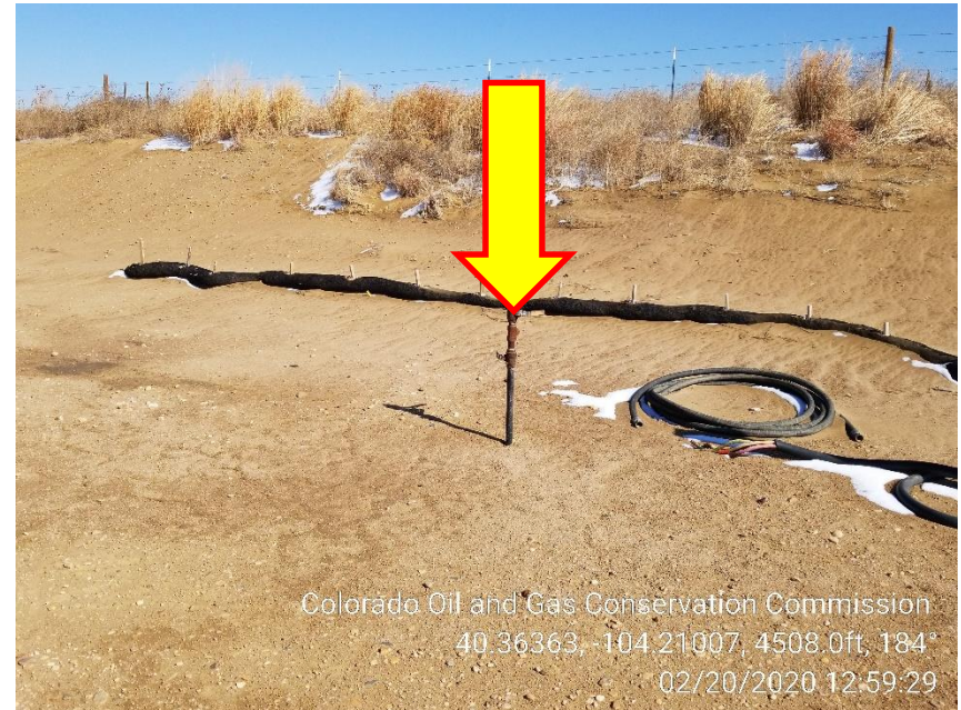
Photo 4 – Unmarked Risers on the Eastside of location
