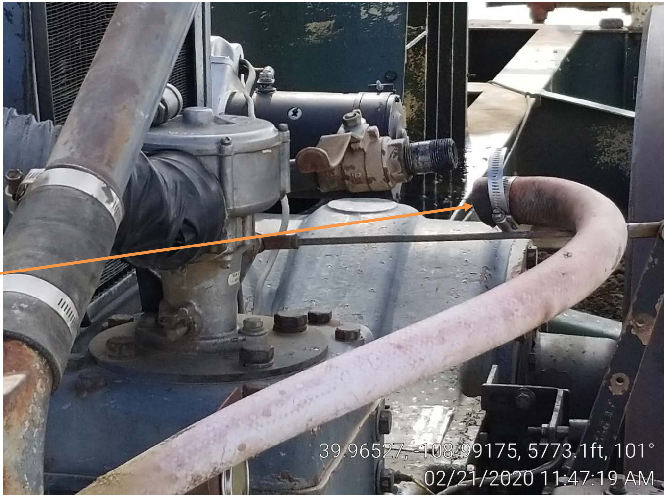
Photo 4. Gas leak at pump jack motor.
