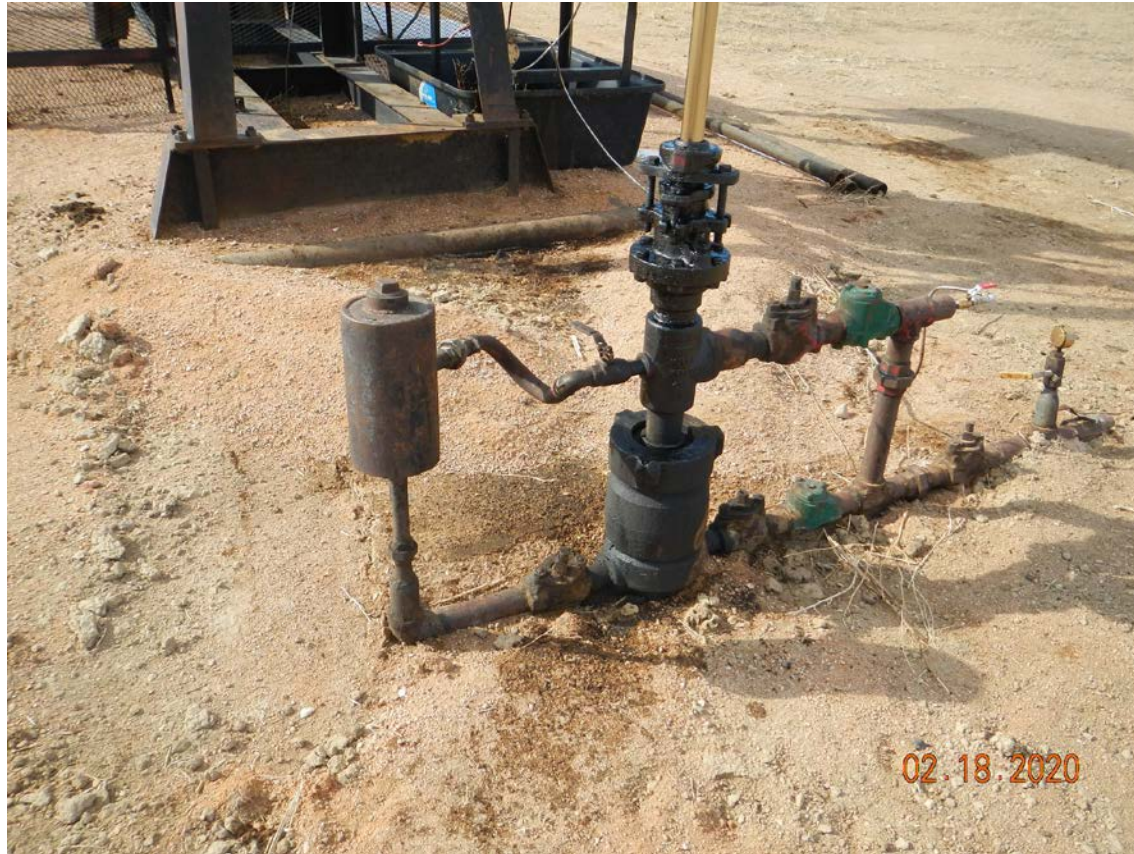
Photo # 1 – Oily soil at wellhead and north of wellhead
