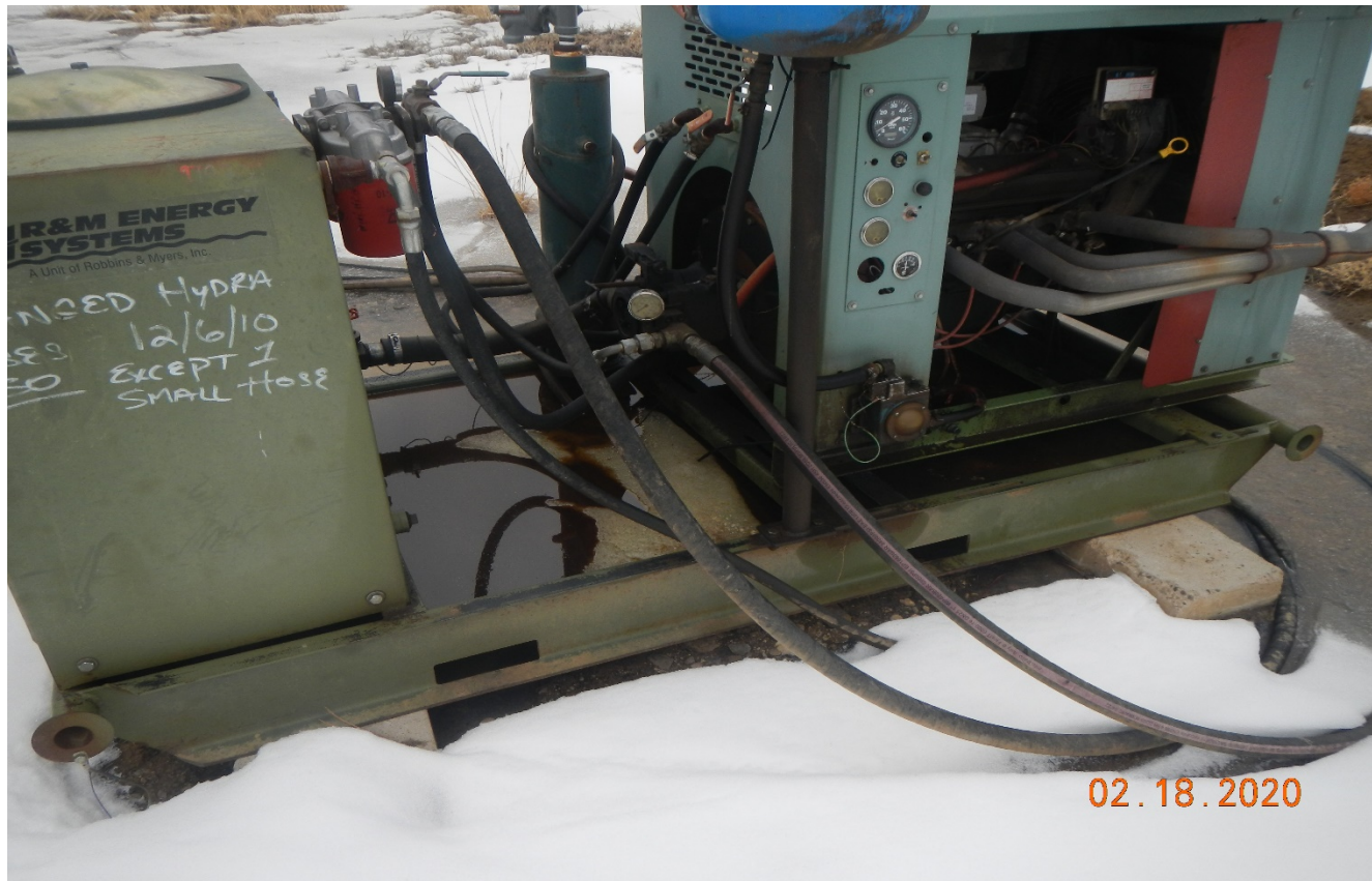
Photo 2. There is oil in the engine skid that needs to be cleaned up.
