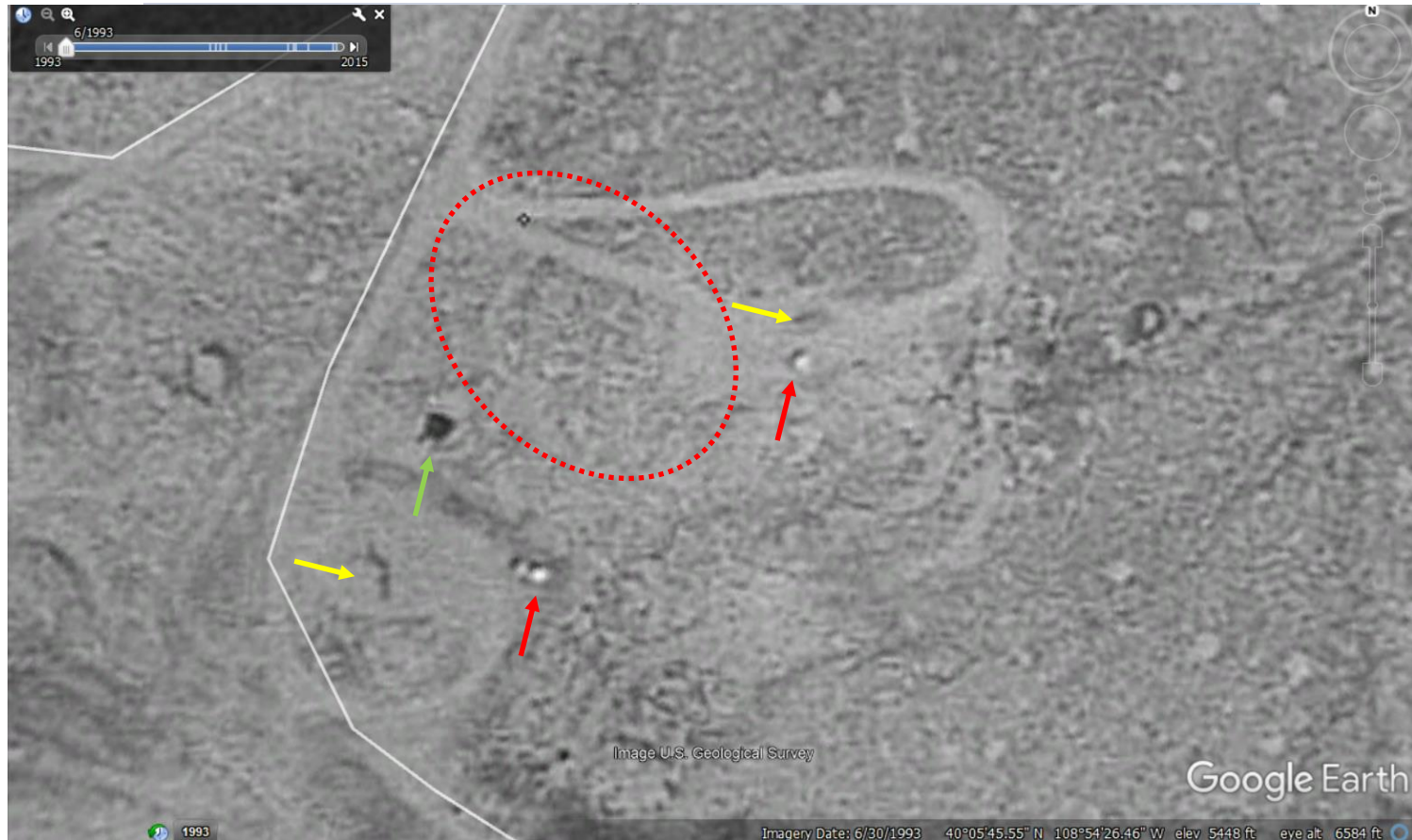
Photo 2: Google Earth Aerial Imagery dated 6/1993. The only active wells at this point are the Emerald C 125 (103-4008) and the Emerald 275 (103-09135). Arrows (yellow) show well locations (yellow), pit (green), and tank batteries (red). Note no equipment is evident within circle at this time
