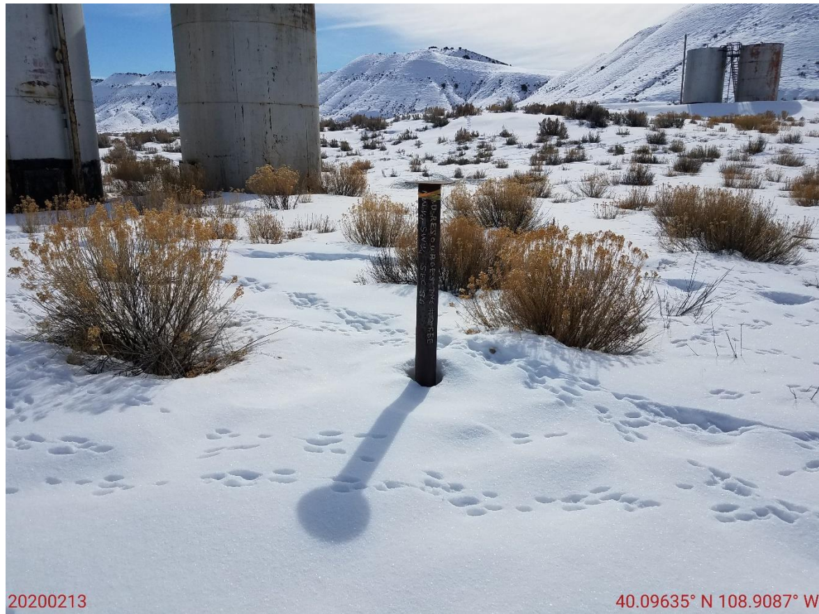
Photo 13: Photo of a dry well marker for the D&D Resources Inc's "Emerald C DCD #2" well. Well was SPUD 7/14/1994 and did not produce. Inspection dated 11/20/98 documents a dry hole marker on the Location with comments "No tank battery equipment", "General Housekeeping-OK", "OK to release"; No surface equipment appears to have been documented.
