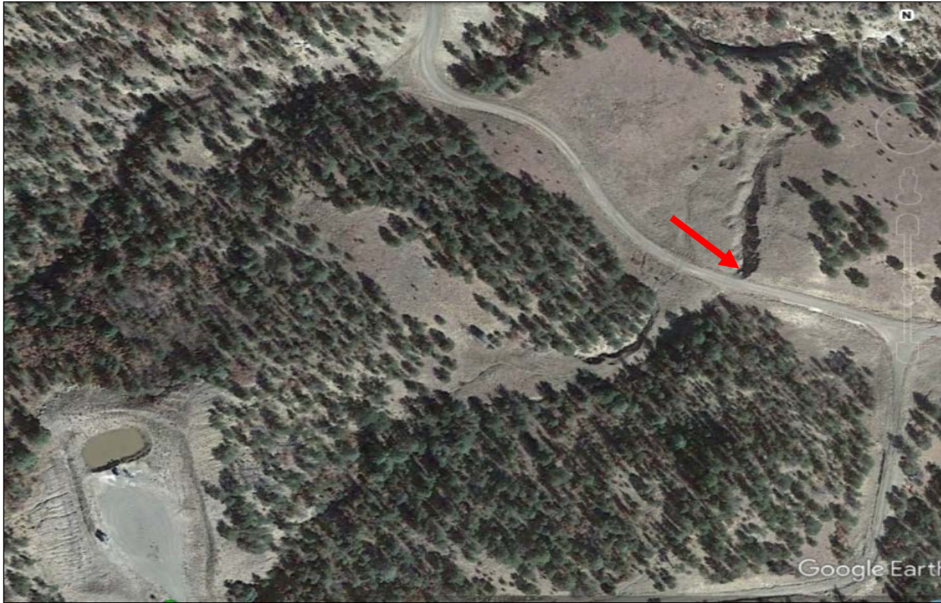
Photo 4. Aerial image shows erosion identified in the previous photo at red arrow. It appears there is stormwater runoff from the Crazy Woman 32-27 location contributing to erosion.
