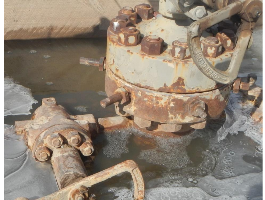
Bubbling in cellar around GM 44-20 well head.
