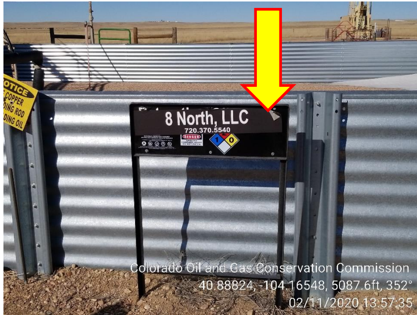
Photo 7 – Missing Capacity Label
