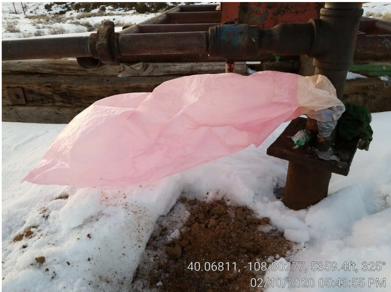
Photo 5. Gas measurement bag attached to well head after 125 minutes.
