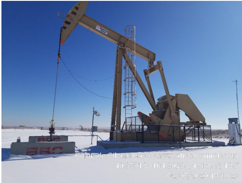
Photo 1 – Pumping Unit, State 5-62-27-0857BH
