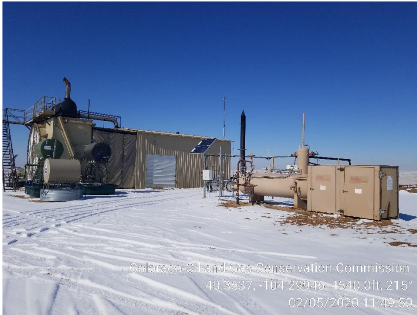
Photo 5 – Compressor and Separator
