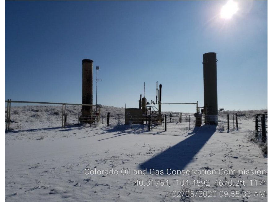
Photo #3 Separator & ECD's
