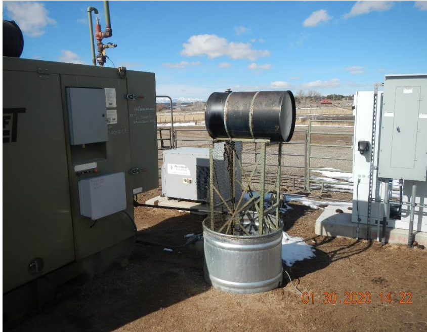
Lube oil container on secondary containment.
