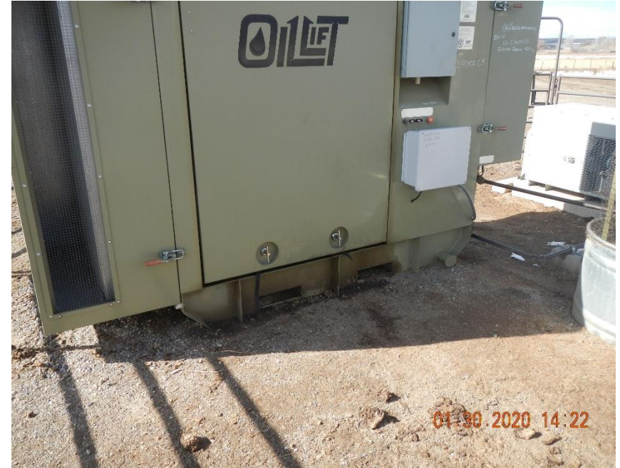
Lube oil staining on equipment and surrounding gravel.
