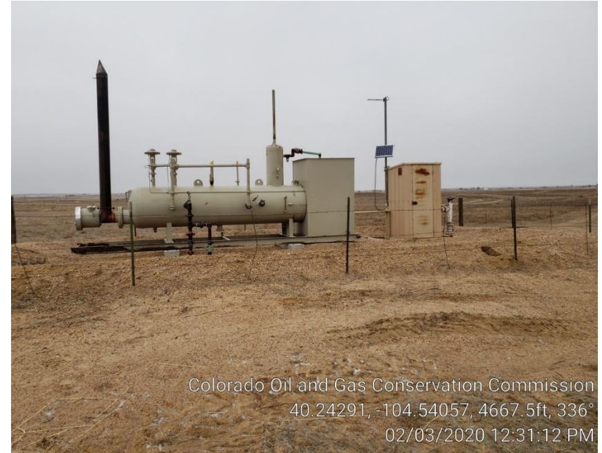
Photo #2 Separator & Meter Run
