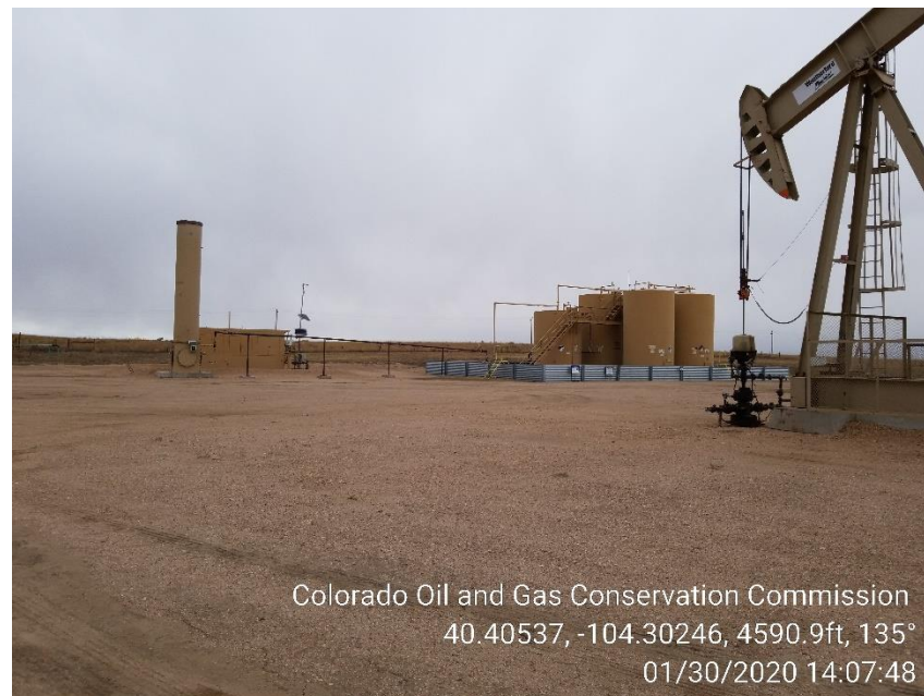
Photo 2 – Tank Battery
