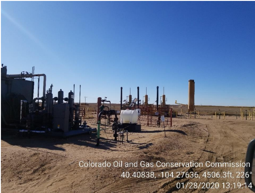
Photo 3 – Separators and Compressors
