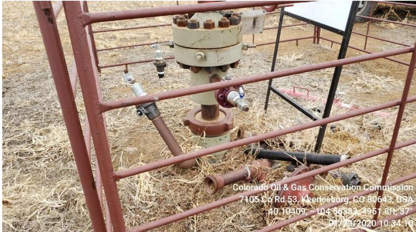
**Photo3 Unused equipment partially buried around WH
