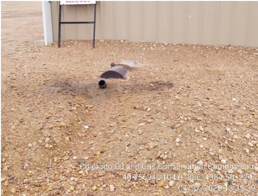
Photo 3 – Stained Soil at Exhaust
