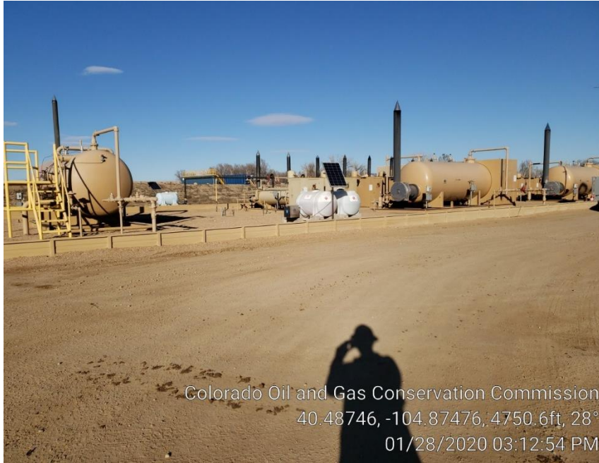
Photo #2 Separators & Heater Treaters
