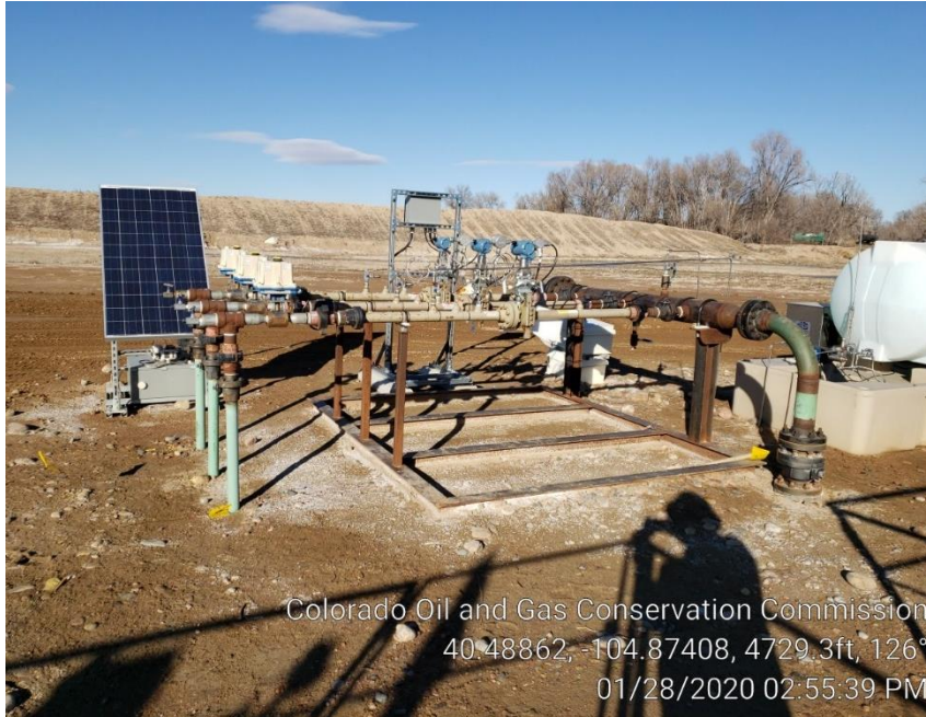
Photo #8 Gas Lift for North Production Wells
