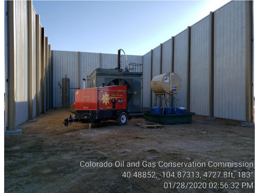
Photo #9 Gas Lift Compressor & Rig Heater
