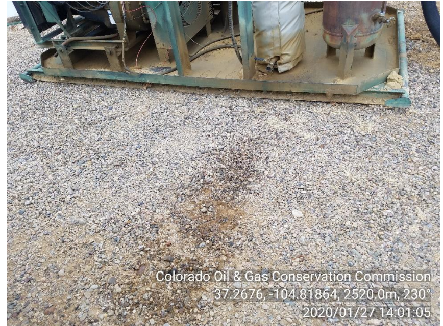
PHOTO 4: APPEARS THAT FUEL GAS SEPARATOR IS BEING DRAINED ON LOCATION LEAVING AN AREA OF IMPACTED SOIL NEAR COMPRESSOR. CAPTURE AND PROPERLY DISPOSE OF ANY OILY WASTE FROM FUEL GAS SEPARATOR WHEN IT IS DRAINED. PROPERLY DISPOSE OF IMPACTED SOIL CA DATE 2-1-20
