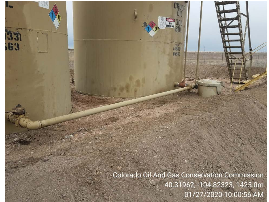
Load valves and stained soil on 1/27/2020
